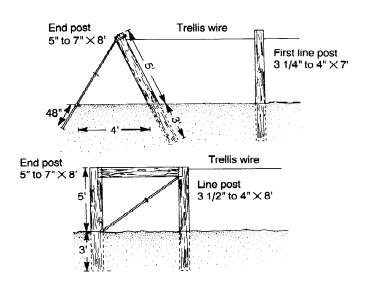
**Figure 1.** Dimensions for the end post construction for a grape trellis that can be used for either midwire or high-wire cordon training systems.
